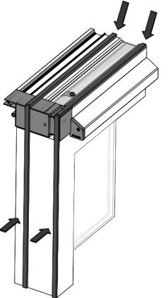
With the Tronic version, pass the cable through the conduit. Tilt the window into the opening.
